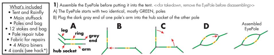
C & D) Flex the two ends together and put the other arm into the socket <<to take the EyePole apart, pull the dark gray ends out of the hub>>
